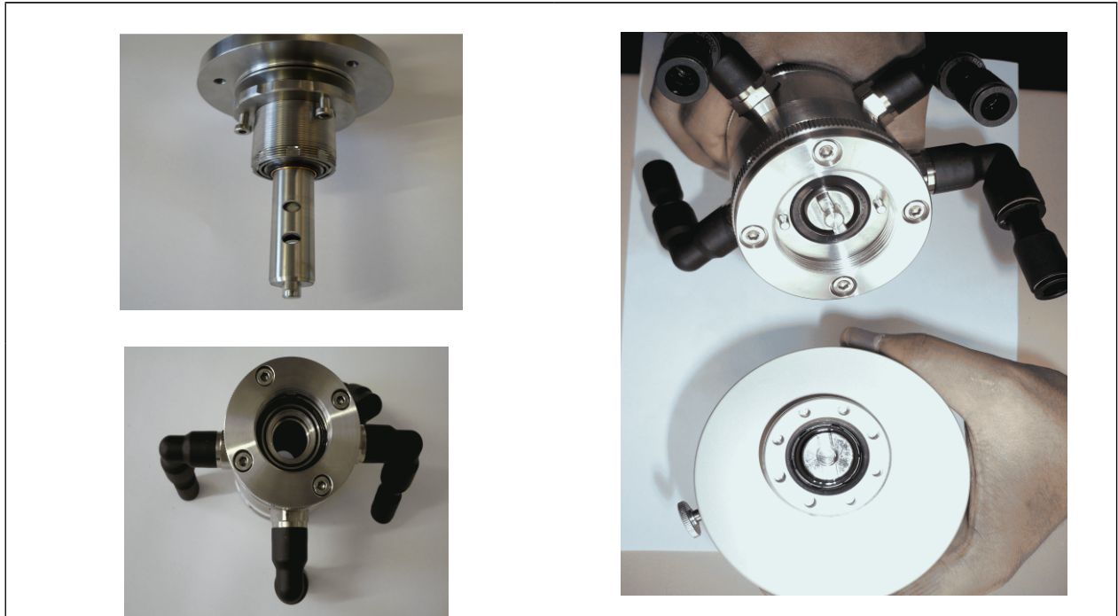
Fig. 7 Installation of water unit to shaft
