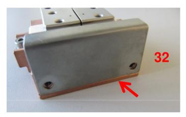
32) Place the anode shield on its position.
