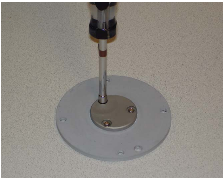
FIGURE 6.12 Loosen and Remove the Gas Distributor Plate Hardware.
