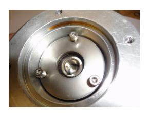
4) The one way clutch should slide out of the clutch housing, again inverting the assembly and tapping the face is all that's required to release the clutch..
