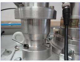
3) Remove the three screws that hold the top of the one way clutch assembly into the main clutch body. Then remove the top of the clutch top plate. You may need to turn it upside down and gently tap it on the table to separate.
