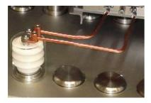
The scan connection is made at the front of the gun. The Temescal scan connection is via 4 wires, the Ferrotec scan control only uses 3 wires. To connect the Temescal scan coils, simply make a common -volts connection by connecting one terminal of each scan coil to the -volts of the Ferrotec scan coil feedthrough. This is easily achieved at terminals of the gun itself.
