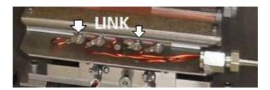
The X and Y scans are identified by the etching on the coil surround, the signals from the Genius can be inverted to ensure the beam is pushed in the correct direction in both the X and Y direction.
