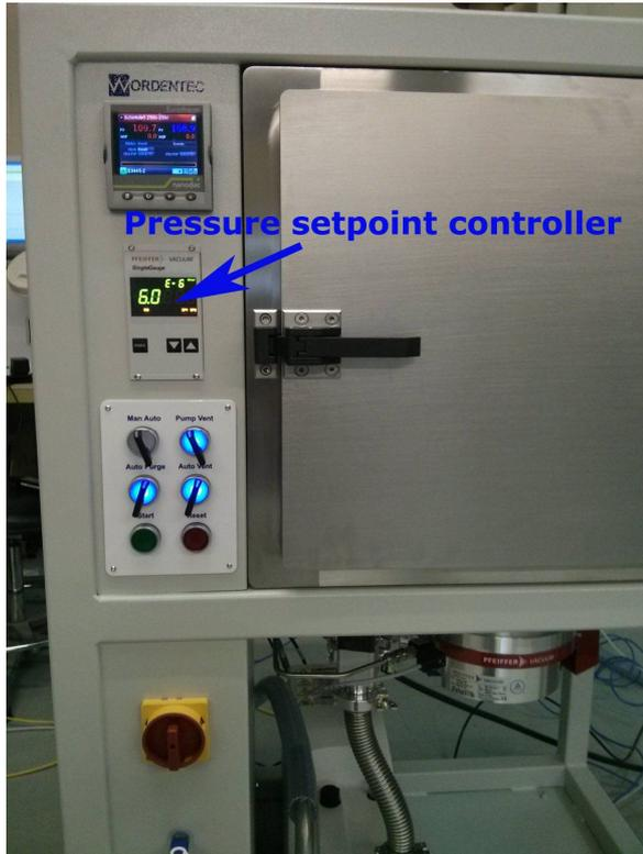
The system uses two pressure setpoints that are defined in the TPG vacuum gauge controller. These setpoint relays can be set for any pressure level within the scope of the gauge connected. Some caution should be used if altering the settings of this instrument as the process will not proceed without vacuum gauge input. The setpoints configured here are not the start process setpoint. This is configured in the nanodac controller.
